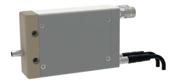
The EMSV electric spray valve is an electromagnetically controlled applicator for the processing of materials such as sealants, adhesives, greases, paints, oils and many other media. The spraying process can be carried out as either an intermittent or continuous process.
