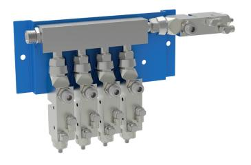
The paint changing unit can handle one medium or switch between several media (depending on the version). It also has an extra connection for a flushing agent, which is used to clean the pipeline prior to each medium change. The valves are each controlled by an external 5/2 way valve (not included with delivery).
