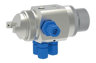
The spray valves of series GF/4 and GF/4 HVLP are pneumatically controlled spray valves. They are suitable for spraying colours, paints, release agents, oils, glues, adhesives and other fluids. Depending on viscosity of fluid different nozzle dimensions are available.
