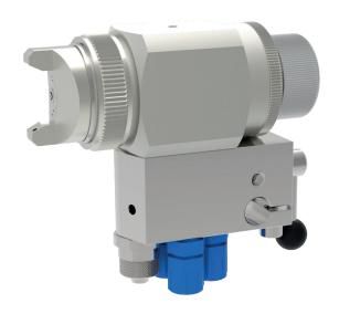
The sprayvalves of series GF/5 with quick release adapter are designed for spraying paints, colours, release agents, oils and other fluids. Depending on viscosity of fluid different nozzle sizes are available. Depending on position of regulation of spray jet, this valve sprays from round- to flatspray.
