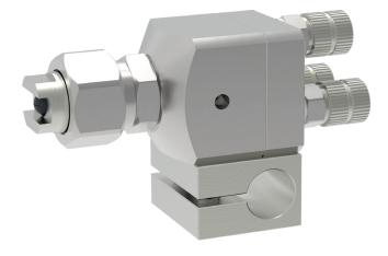
The KA-2 / AIRLESS automatic spray valve is an airless atomising spray valve. The material to be processed is supplied to the device at high pressure. A special AIRLESS nozzle is responsible for the atomisation.
