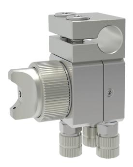
The automatic spray valve KA-2 is, because of it's low weight and the small measurements, ideal for all spray jobs in machines or robots. This spray valve can be used for all thin fluids, f. i. release agents, oils or colours. Depending on air cap this spray valve sprays in flat or round spray. Depending on viscosity of fluid, the application can be adjusted individually via nozzle dimension, atomizing air pressure and material pressure.
