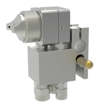
The sprayvalves of series KA-2 with quick release adapter are designed for spraying release agents, oils, paints and in version KLS also for glues and adhesives. Depending on viscosity of fluid different nozzle sizes are available. Depending on air cap this valve sprays in round or flat sprayjet.
