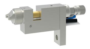
The spray valves of series MFS are pneumatically controlled spray valves. They are suitable for spraying release agents, oils, colours and in version MFS/KLS also for glues and adhesives. The control of valve will be done via external solenoid valves or mechanical valves. The supply of fluid will be done via pressure tanks or pumps.
