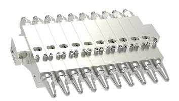
The bead application heads are used for application of multiple beads from one overall head. Different hole gauges can be produced between the nozzles. The number of modules for application is variable. The individual modules on the bead head can be activated jointly in the desired groupings. Each individual module can also be activated separately.
