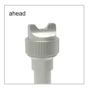
The D12 nozzle extensions have an outer pipe diameter of 12mm. They consist of an inner pipe for the medium, a central air pipe and a horn-shaped air pipe. The special characteristic of these extensions is that they can generate a controllable spray jet (round and flat spray pattern). The D12 extensions are available for all guns/automatic spray valves with integrated round/flat spray pattern adjustment (e.g. W3FZ-Duo R/F, S 947, MKD-IS R/F, GF-3).
