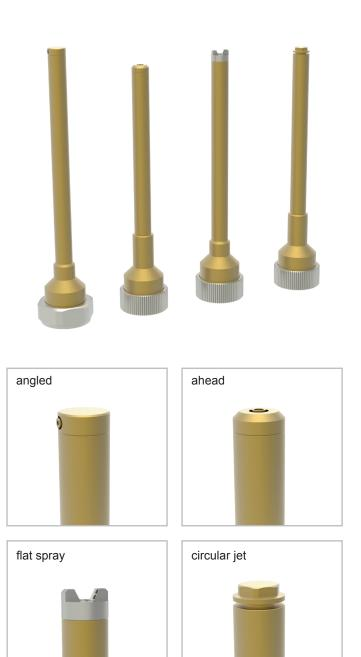
The nozzle extensions of the D8 series have a pipe diameter of 8 mm. They give the opportunity to solve application jobs by their small dimensioned construction, especially for the installation in machines or robots because of very low space requirements. Also suitable for spraying into very small moulds or through small holes.
