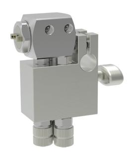
The spray valves of series MSV with quick release adapter are designed for spraying release agents, oils and other thin fluids. Depending on viscosity of fluid different nozzle sizes are available. Depending on air cap this valve sprays in round or flat spray jet.
