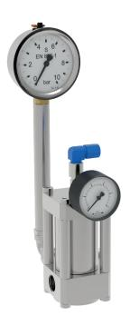
The SCHÜTZE material pressure regulators are used for regulating fluid pressures. Their function corresponds with pressure reducers. The maximum outgoing material pressure can not be higher than the incoming material pressure. The air pressure (in drawing marked with "Luft") determines the outgoing material pressure (marked with "Aus").
